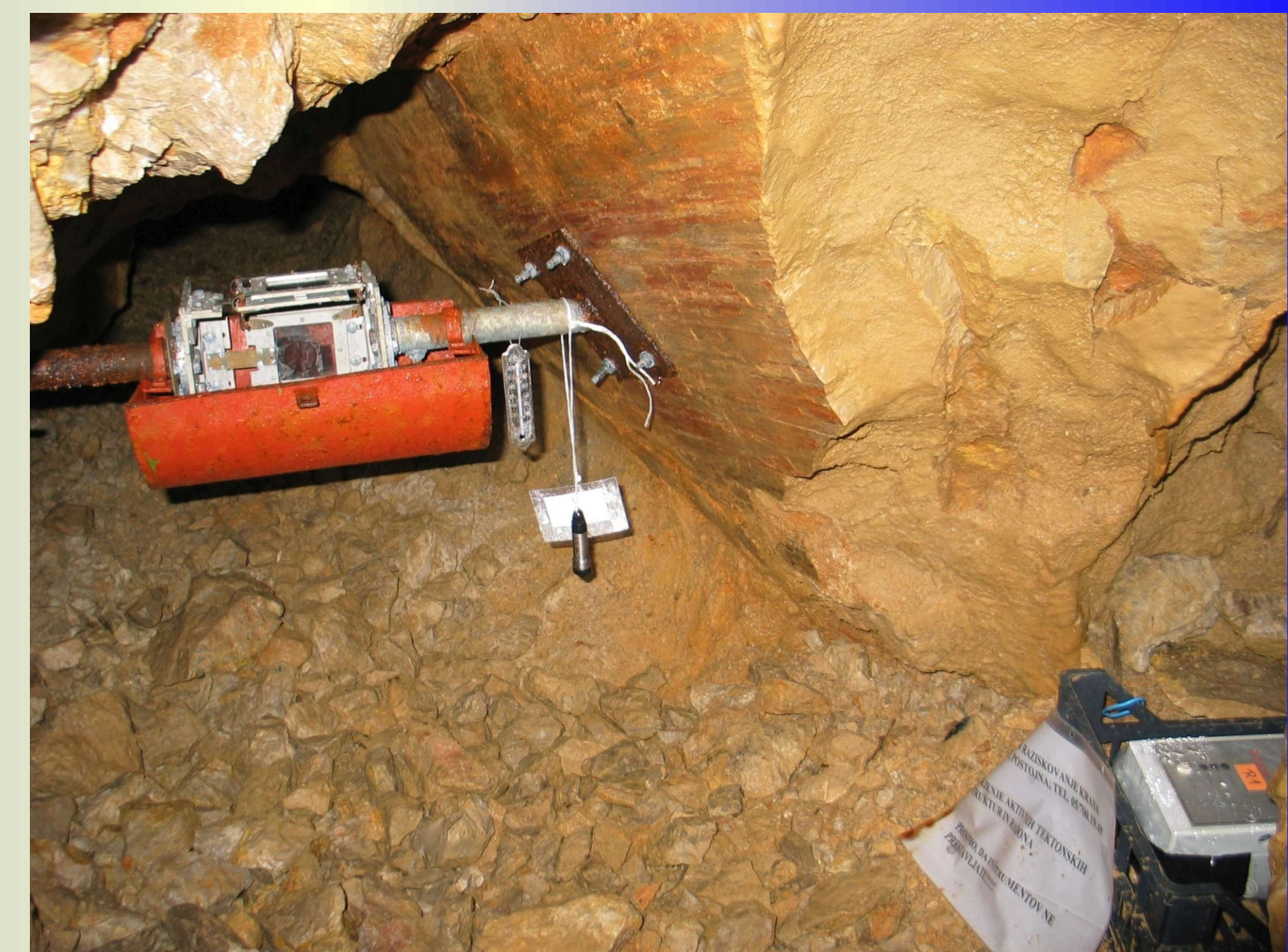
Micro-displacement monitoring with TM 71, radon monitoring and cave air T monitoring in Lepe Jame (Postojna 2).
